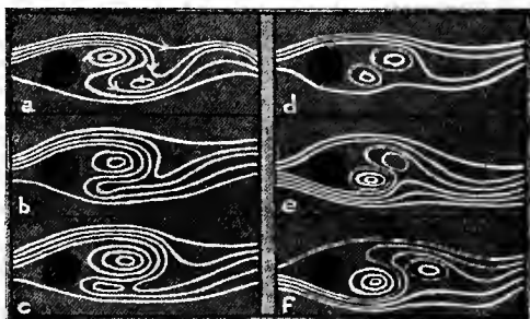
FIG. 58.—Six successive drawings, a to f , showing how air-whirls are formed, first on one side of a wire, then on the other, as the wind blows past it. The black circle is a section of the wire.
