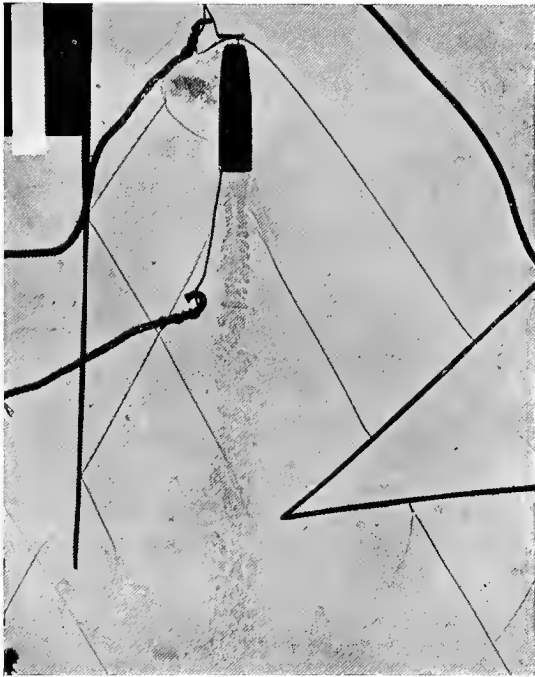
FIG. 87.—Bullet from Martini-Henry rifle photographed while in flight by C. V. Boys. Two V-shaped ripples are clearly seen, one coming from the nose, and one from the stern of the bullet.
