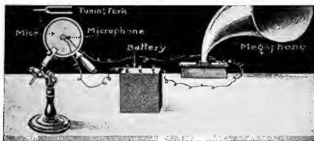
FIG. 82.—When the tuning-fork is held symmetrically at the edge of the disc, very little sound comes from the megaphone. But when it is held to one side, the response is loud.
