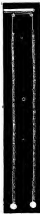
FIG. 33. — The two springs are connected by a fine cord running over two aluminium wheels mounted on ball-bearings. The white balls suspended from the springs are quite light.
