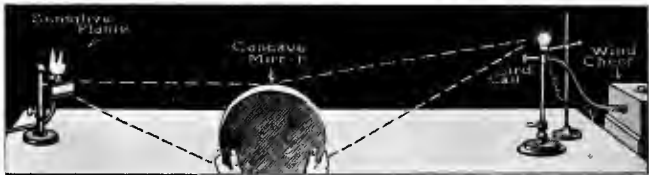
FIG. 16.—Reflection of Sound by Concave Mirror. The mirror reflects and concentrates the light from the lamp (above the bird-call) upon the piece of white paper, and at the same time reflects and concentrates the sound from the bird-call upon the sensitive flame.
